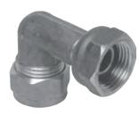
Swivel elbow 90°. 15mm compression copper to ½" BSP female iron connection end. SANS 1067-1.
