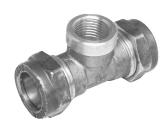
Copper to copper to female iron reducing Tee. 22mm compression copper to copper connection ends on run, 1/2 "BSP female iron branch.
