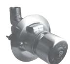
Undertile metering stop tap with non-hold open feature, flow controller and stainless steel wall flange. Brushed chrome finish. Flow cycle 1-20 secs. 1/2 BSP Male connection ends. SANS 1808-9.
