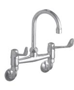
Elbow action,  $\frac{1}{2}$  turn ceramic disc, wall type mixer with swivel outlet.  $\frac{1}{2}$  BSP fixed male connection inlets with 178mm centres. SANS 226 TYPE 2.
