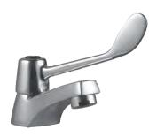
Elbow action pillar tap square type with blue indice. ¼ turn ceramic disc. ½ BSP male connection inlet. SANS 226 TYPE 2.
