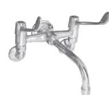
Elbow action, ¼ turn ceramic disc, wall type mixer with fixed outlet and reinforcing back plate . ½" BSP fixed male connection inlets with 178mm centres. SANS 226 TYPE 2.
