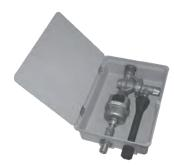
400kPa Master meter box consisting of 1 x PA3.132 pressure control valve, 1 x ¾" ball cock, funnel, GRP box with lid, 2 x PB6.303 vacuum breakers and 1 x Kent water meter. 34" BSP male connection ends. SANS 198.
