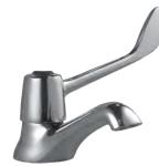
Elbow action pillar tap with raised nose and blue indice. 1/4 turn ceramic disc. 1/2 BSP male connection inlet. SANS 226 TYPE 2.
