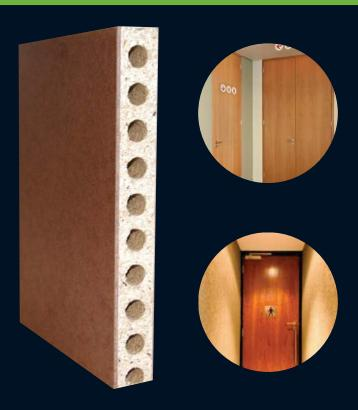
Now you can get fire protection with the added benefit of acoustic insulation from one door. Trucore fire rated doors are manufactured for a guaranteed and proven 30 minute fire protection and up to 34DB sound insulation making it the obvious and most economical choice. Trucore 30 minute fire rated doors are manufactured from a tubular particle board core of 354kgs/m3.
