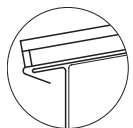
Eaves termination, standing straight (only recommended for areas where aesthetics are important)
