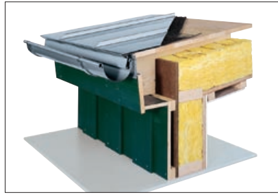
Ventilated roof structure 2 with ventilated supporting structure, without full rafter insulation and with a structured underlay
