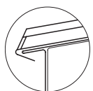
Eaves termination, standing diagonal
