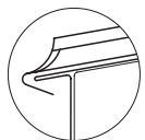
Eaves termination, standing round (favoured solution)
