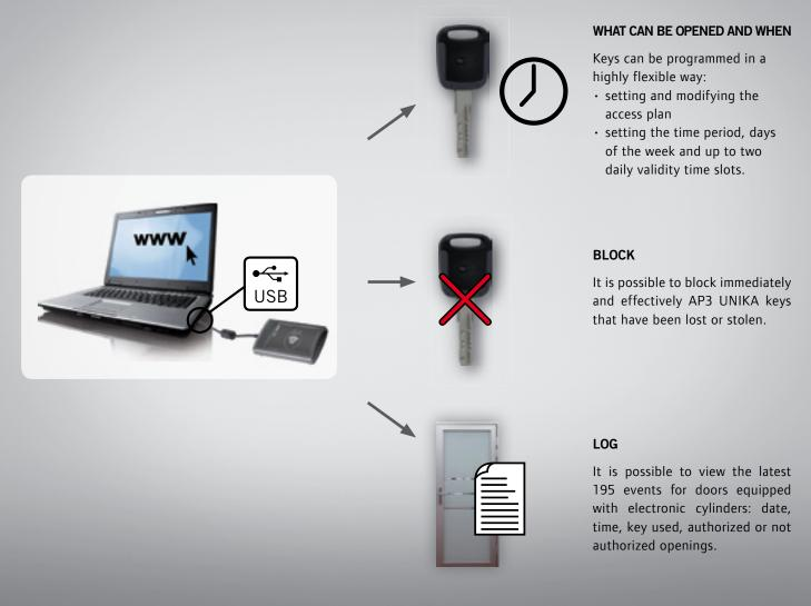
AP3 UNIKA combines the advantages of software management with an easy-to-use, web-based platform. It offers immediate operational design: no management software is needed; it is enough to connect to a PC the reader contained in the AP3 UNIKA kit and go to the website **www.cisa.com/authenticard**.
