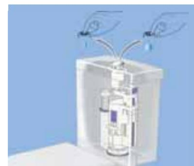
**Dual Flush.** With the two-volume technology (3 or 6 liters), a household of four can save more than 40,000 liters of water/year. Press the small button for the small flush volume. A minimum flushing volume washes away liquid waste in a clean and hygienic manner. If you wish to use the full water volume, simply press the large button.
