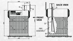
Note: A stand is available for floor mounting (as shown above) & for pitched roof installation with pitches of more than 8° & less than 30°. All dimensions in mm.
