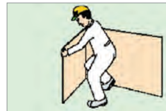
Snap Lafarge Plasterboard and cut other side of paper
