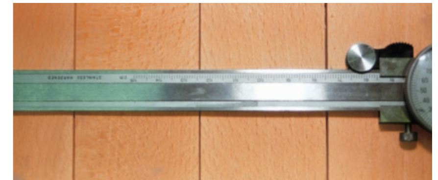
SikaBond adhesive after alternating climate cycle
