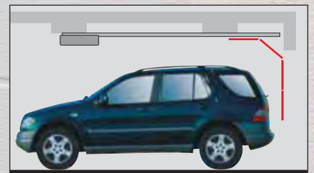
Reduced headroom requirement = 115 mm
